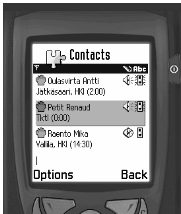
Figure 4. ContextPhone is a context/information-enhanced contact book for mobile phones. Next to each contact, the phone automatically updates information on how recently the phone has been manipulated by the person (the hand icon on the left), his/her current location (and time spent there), and phone profile (audio and vibration alarms on/off).
