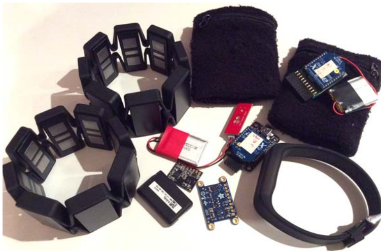
Figure 1. Some of the wearable devices used in prior research. Clockwise from the bottom-left corner: Myo armbands, Sense/Stage controllers with wristbands, Axivity WAX9 with silicone wristband, Adafruit 9-DOF IMU Breakout, FreeIMU v0.4.
