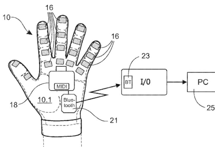
**Figure 1.** A diagram of the KAIKU Music Glove with a musical instrument digital interface (MIDI) and Bluetooth (BT) connected to a personal computer (PC). The KAIKU Music Glove generates musical data through a glove embedded with touch sensors and electronic units. It connects via Bluetooth or Universal Serial Bus (USB) to a host device (i.e., laptop or personal computer) to produce musical sound.
