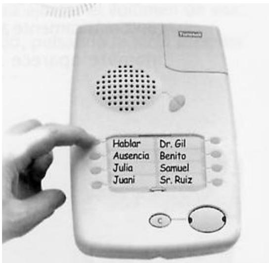
**Figure 1.** Fixed Telecare Device<sup>1</sup>.
