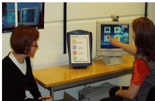
Figure 7. Industrial designers from the University of Lapland experimented with concepts and UI features of videophones by constructing a realistic wooden mock-up.
